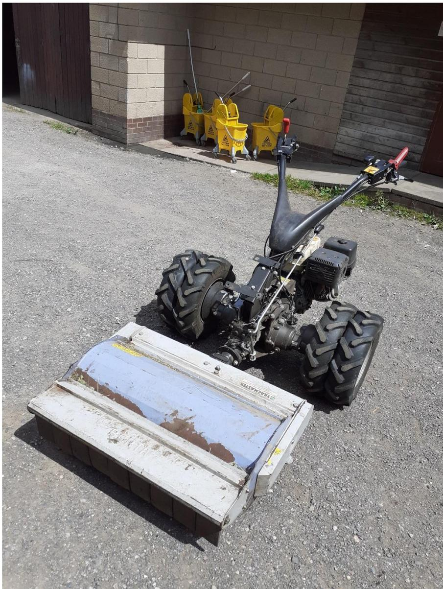
The BCS flail mower used for roadside verge cutting
